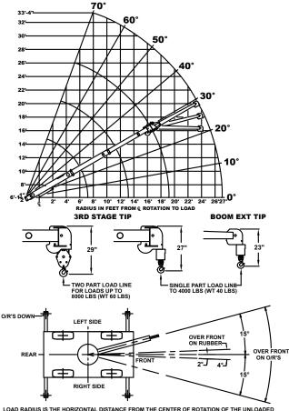
LOAD RADIUS IS THE HORIZONTAL DISTANCE FROM THE CENTER OF ROTATION OF THE UNLOADED CRANE TO THE VERTICAL LOAD LINE WITH THE LOAD APPLIED.
